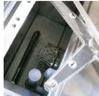
Tank with rounded edges and slanting bottom for the highest hygiene.
