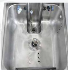
Some areas around the **washing tank** have the purpose to gather all dirty materials and to guarantee the proper working of the washing cycle's phases. A frontal filtered zone cathces the superficial dirt; a second backward zone guarantees the correct filling levels' functioning.
